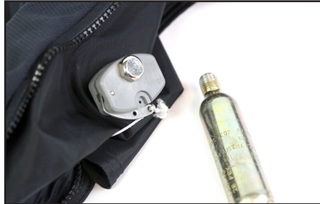
With CO 2 cartridge removed, test proper function of actuator. If needed lightly lubricate with Krytox.
