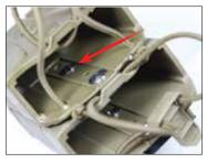
Connect the top holes with the screws and using the hole indicated above, attached the second screw.
