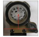
To attach compass, insert light switch into hole. Reattach screws. Red reference line should be perpendicular to individual when in use.
