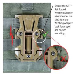
Once the GRT™ Reinforced Webbing Adapter tabs are fed into the top row of MOLLE, pull the adapter down and into the Webbing Adapter Lock. The GRT™ Reinforced Webbing Adapter should snap into the Webbing Adapter Lock indicating that it is secured.
