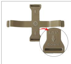
The orientation of the MBS dictates what belt width the adapter will accept. Belt width markings can be found on vertical members of the MBS. The word "DOWN" and a downward facing arrow with the respective belt width indicates what belt width the adapter has been configured for.
