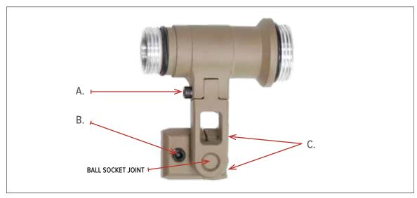
Screw A (x1) locks the flashlight body in left or right side of the helmet orientation. 1/16" Hex screw.
